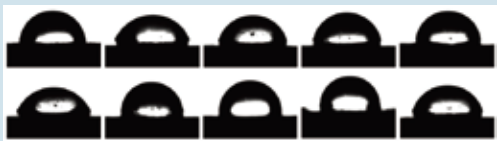
Image of water droplet on untreated zirconia surface
