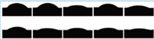
Image of water droplet on STM-treated zirconia surface
